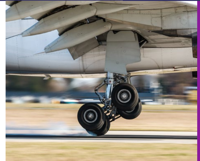
Electric brake actuators allow for lighter aircraft
