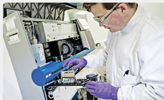
Calibration verification of a module in the Cedex Bio HT (Roche Life Sciences). The Cedex Bio HT measures a range of cell metabolites and ions from cell culture media to improve understanding of critical process parameters in cell expansion and differentiation
