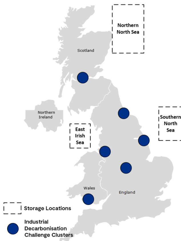
Figure 3: Location of Potential CO 2 Storage Facilities in reference to UK Industrial Clusters.
