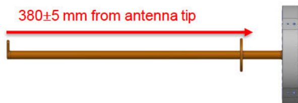
Figure 5: Gold Plating Location
