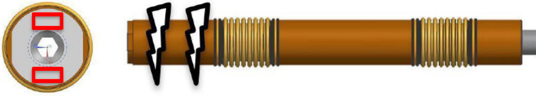
Figure 10: Air Inner Conductor S/N location
