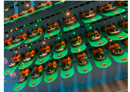
Coins cells being tested to understand their performance after remanufacture from recycled material via the organic selective phased leaching technology.
