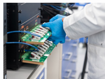
FutureCat researcher loading a coin cell onto an instrument for electrochemical characterisation.
