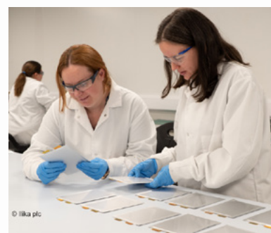
Solid-state battery pouch cell testing at Ilika. Photo courtesy of Ilika.
